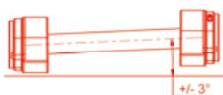
The construction permits a misalignment of the bearing, of up to  $\pm 3^\circ$
